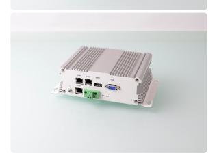
E3845 Quad Core 1,9GHz, 1xDDR3L SO-DIMM socket, HDMI+VGA, 1xSATA 2,5", 2xIntel I211 LAN GbE+Intel I211 LAN(опция), USB 3.0 + USB 2.0 (1A), 9-36V, work t: 0-+50C, storage t: -40-+85C
